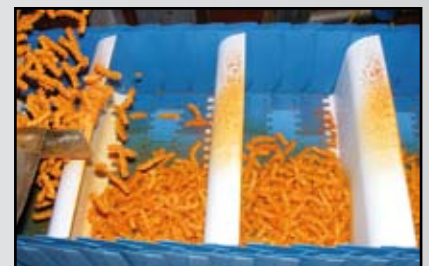
INFEED OF INCLINED CONVEYOR WITH 2010 ISR6
