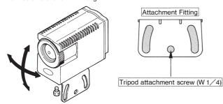
It is possible to angle the product by 45 degrees upward/downward or left/right if the provided attachment fittings are used. The two taps of the attachment fittings are the tripod attachment screws (W 1/4). By screwing the attachment fittings onto the main unit, the product can be attached to the tripod.
