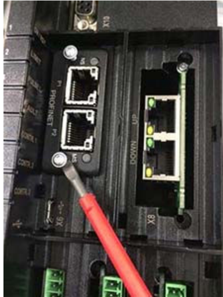
Figure 5-22. Anybus module removal
