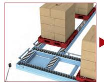
The aim is to sense the target object as it reaches the designated position.
