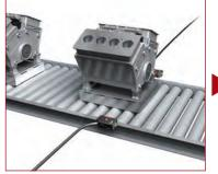
Reflected light passes through gaps in the target object, causing detection errors.
