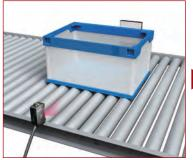
Light passes through semi-transparent target objects, affecting detection consistency.
