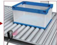
Target is now detected correctly. Note: Highly transparent objects cannot be detected. Check with actual target objects before running a machine.
