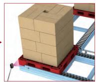
The sensor operates around at this position. Note that the sensing distance can vary by as much as 15% from the set distance.
