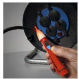
Testing of cable breaks
