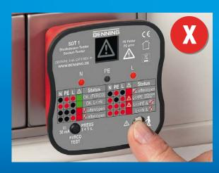
Socket with wiring error, danger to life! External conductor (L) and protective conductor (PE) have been inverted!
