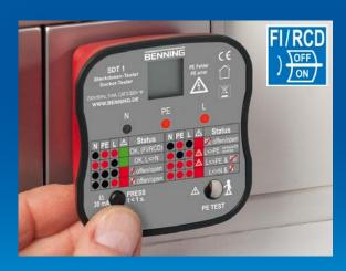
Testing the tripping function of a 30 mA RCD by pressing the FI/RCD TEST key
