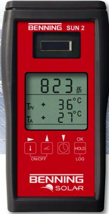
Insolation, PV module/ambient temperature
